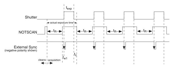
Figure 46. Overlapped Mode where Pulse arrives after Readout
